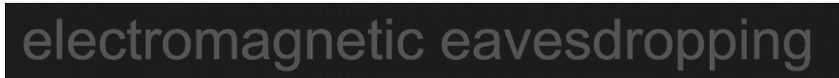
Fig.11. The reconstruct image in base on theoretical sensitive emission corresponds to displayed image from Fig.10 (DVI standard as a source of emission, ClearType smoothing mode of edges).
