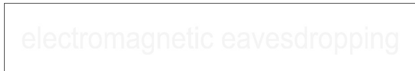
Fig.10. Image displayed in screen including text data in color 245 on the background in color 255 – invisible data.
