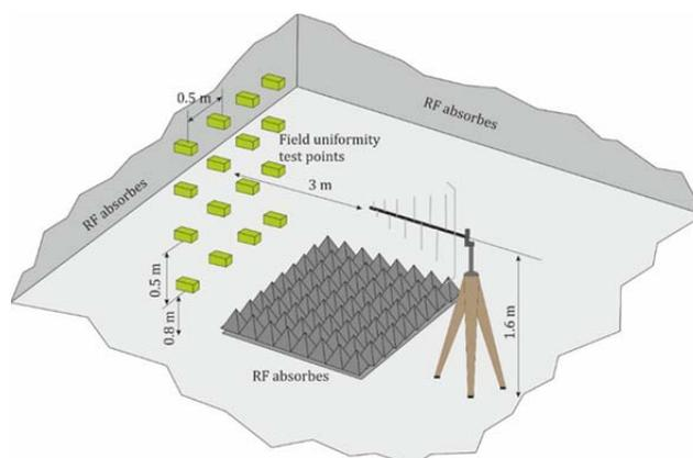
Fig. 2. The test setup for electromagnetic field calibration
