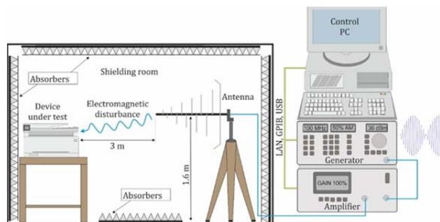
Fig. 3. The test setup to EMC immunity test
