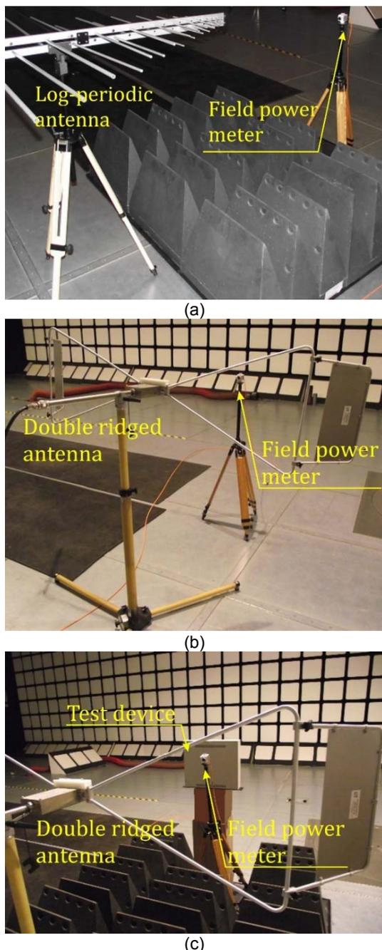
Fig. 11. Measurement setup to check the influence of metal objects on electromagnetic field distribution: (a) with absorbers; (b) without absorbers; (c) with absorbers and EUT
