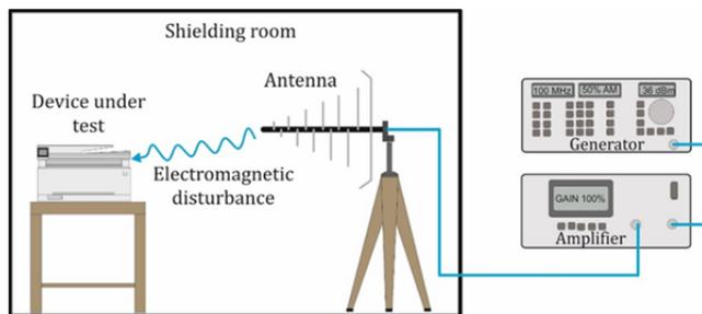
Fig. 1. The general test setup to EMC immunity test
