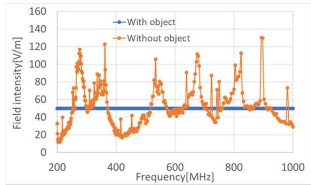
Figure 14. The electromagnetic field intensity indicated by probe both with and without tested object (EUT) by using the same signal power from generator
