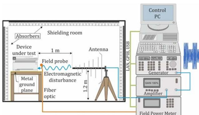
Fig. 4. The test setup for EMC immunity test according to MIL-STD-461G
