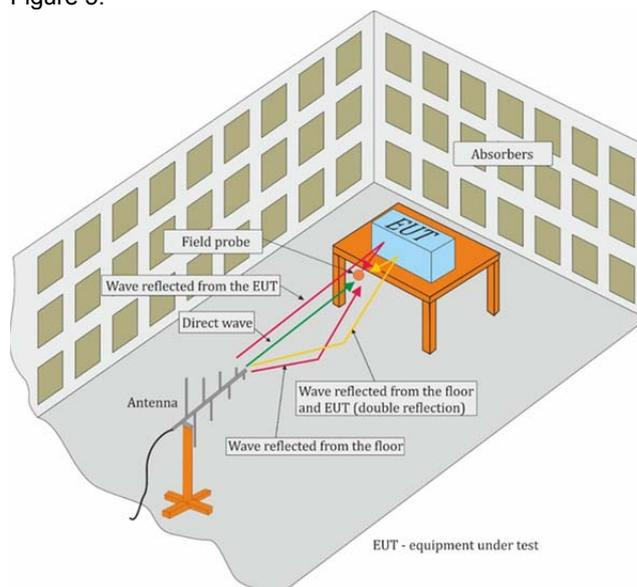
Fig. 5. Visualization of the reflections method (ray tracing) to determine the distribution of electromagnetic field intensity
